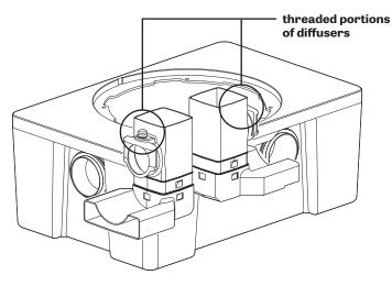
Push the diffuser access coupling onto the threaded portion of each diffuser and set using supplied set screw. Glue the diffuser access riser to each coupling.
