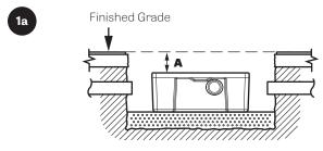
For the interceptor to be safely and properly maintained, dimension **A** cannot exceed 25" (or two FCR1 risers stacked).
