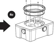
Place riser on interceptor, aligning bolt holes and fasten securely with mounting bolts.
